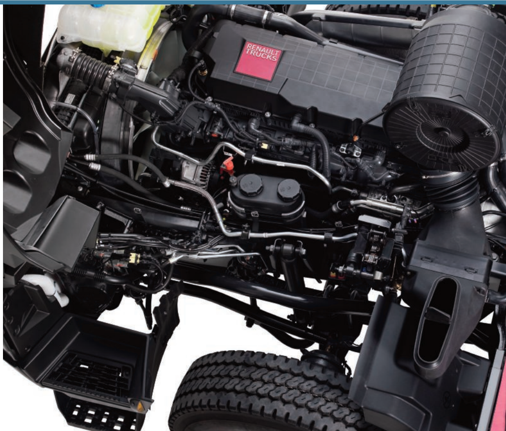
Renault Trucks' Range K Euro 6 drivetrain exposed: ECUs are now distributed around the chassis close to their areas of responsibility
